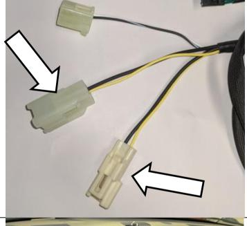
Route the small black plug to the location desired for installation of the gear display. This can go anywhere that the wire will reach and is up to the drivers preference. We suggest the lower right corner of the instrument cluster bezel, the wire may be run between the cluster and the bezel.
