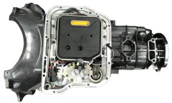
**Important** Check to ensure the steel tube support bracket is still in place and adequately supporting the tube. It may have been moved the previous steps.
