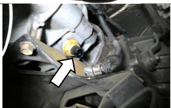
Connect the BD harness to the speed sensor and plug the stock wiring into the BD harness.
