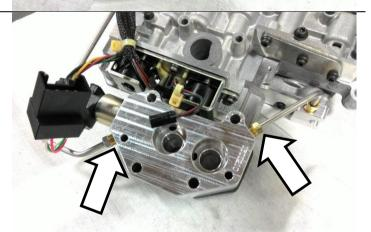
Locate the two solenoids (4617213) supplied in the valve body kit and slide them in the retainer bracket as shown. The plate goes in the top most land of the solenoid.
