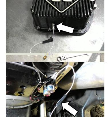
Raise the transmission pan below the transmission and connect the one pin connector from the governor solenoid wiring to the through pan wiring harness.
