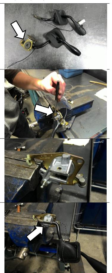
Reposition the spring and bushings for installation.
