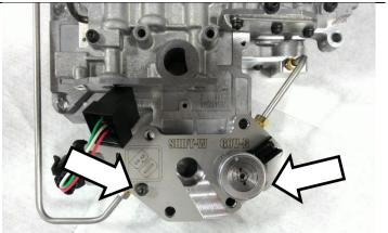
Install your harness and solenoids using the three small T25 screws from the old valve body.
