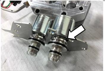
Push the solenoids back down into the governor solenoid housing with the plugs in the orientation shown.
